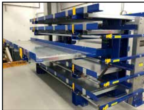
Cantilever Roll-Out Rack Manual Crank stores heavy, large items easily.
